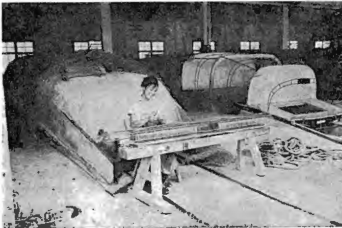
Fig. 2. Precast ferrocement parts for a new boat are made in front of a boat that is curing. Note pit under the hulls and rail tracks used when the completed craft is moved.
