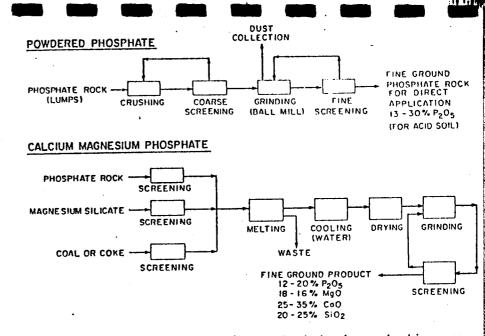
FIGURE VI-3. Small-scale production of powdered phosphate and calcium magnesium phosphate.
