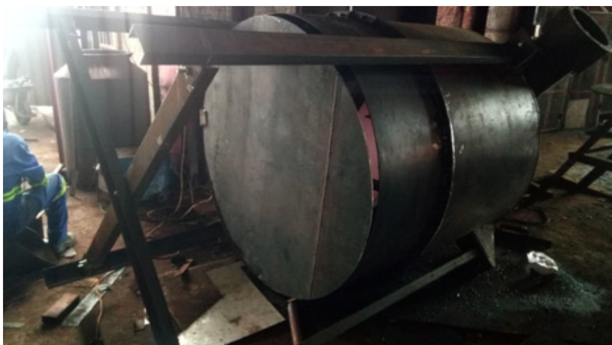
Figure 2: Reaction and ash chamber assembly
