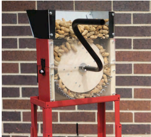
Figure 17. Final Model of Peanut Sheller with Plexiglass front to show operation
