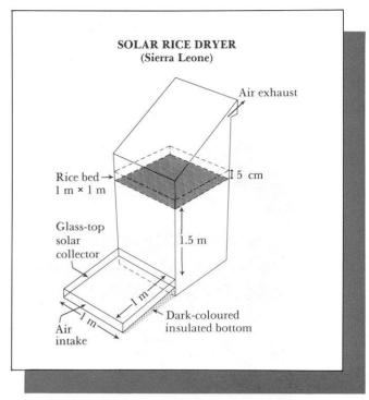
insects. The new design has a simple wooden lid, and a small rear grating to let moist air out.
