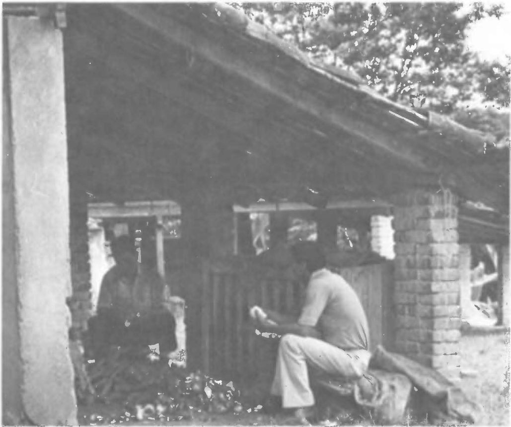
Fig. 3. In this small-scale starch factory, the roots are peeled by hand but not washed beforehand. The ash content, therefore, is likely to be high.
