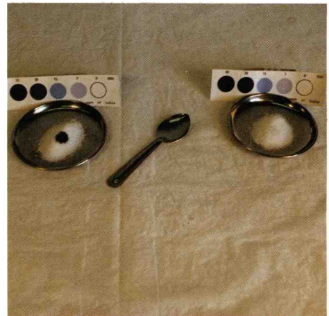
(Chapter 10) - Results of testing with the field kit. The dark spot in the salt on the right shows iodine content, while the salt on the left gave no color, indicating no iodine.
