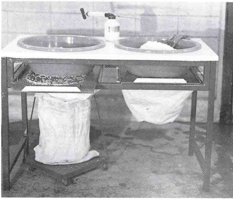
(Chapter 8) - An entirely manual iodization apparatus, with hand spray of an iodate solution, used at the local level (photo: Romsai Suwanik).
