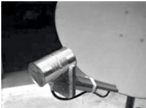
Figure 4.10: Feed horn made from a food can.
