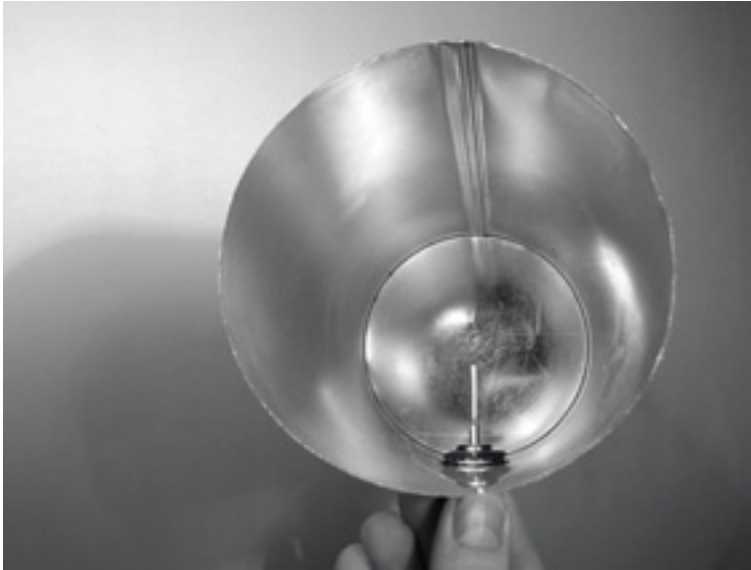
Figure 4.41: Your finished cantenna.
