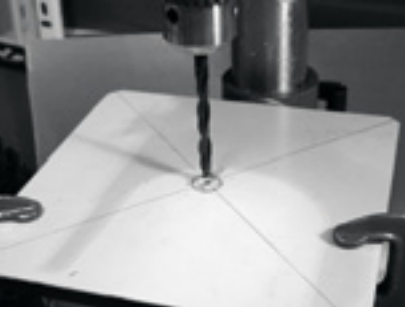
Figure 4.21: Drilling the hole in the metal plate.
