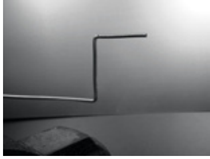
Figure 4.16: Bend the wire into a "Z" shape.
