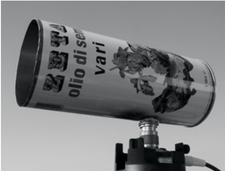
Figure 4.32: The finished cantenna.
