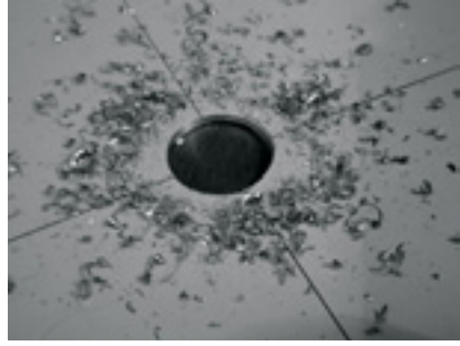
Figure 4.21: Drilling the hole in the metal plate.
