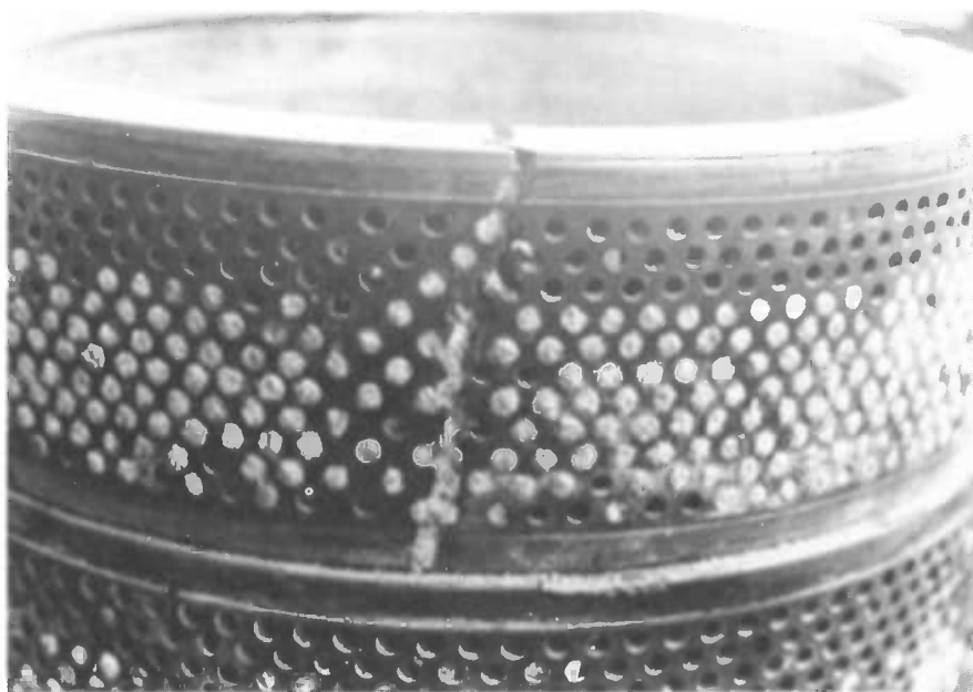
Fig. 5. Broken dies of a presser.
