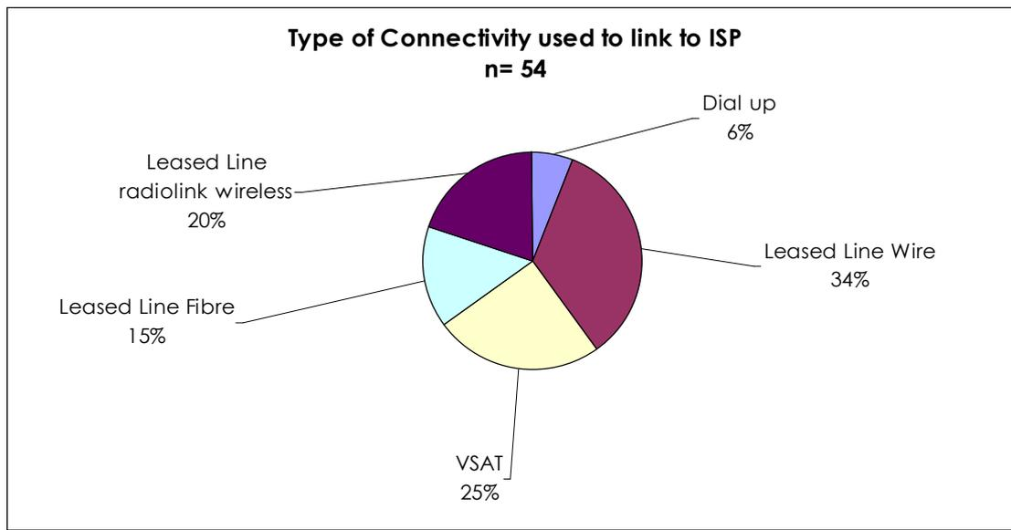
From the above chart it is evident that the majority of the sampled higher education institutions use terrestrial based leased lines for connectivity purposes with satellite (VSAT) coming in second place. In particular 69% (64% in 2004) use terrestrial leased lines (wire, fibre or radio link) for connections to their ISPs, while 25% (29% in 2004) use VSAT. On a downside note, 6% (7% in 2004) of the institutions still rely on dial-up connections.
