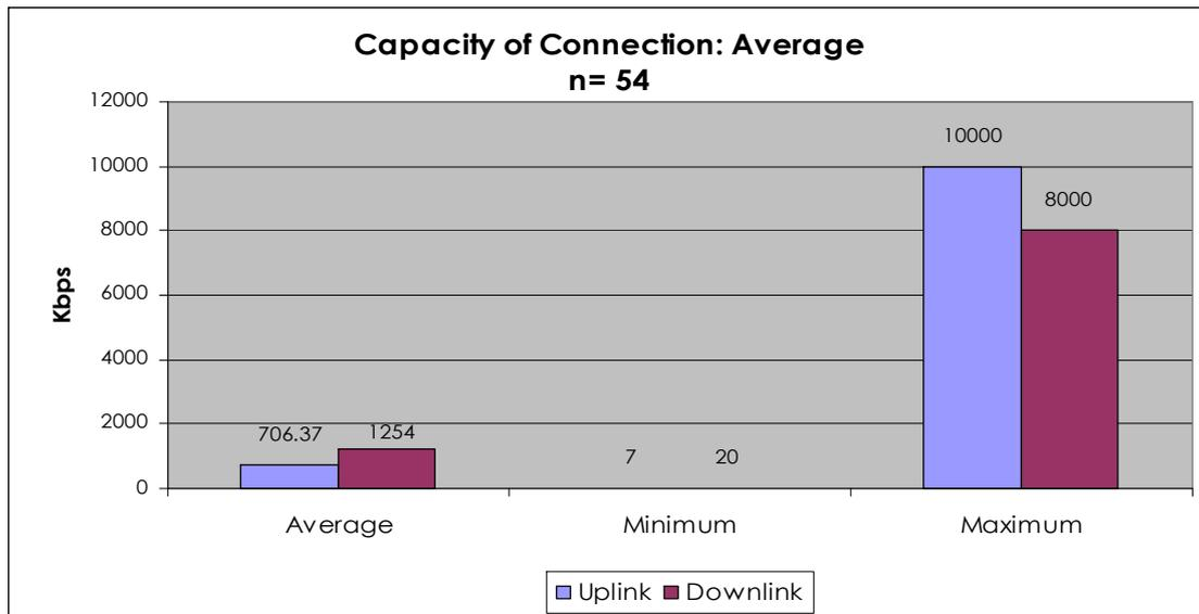
The chart shows that the average bandwidth reported for the uplink and downlink is 706 and 1254 Kbps respectively. Highly notable is the wide gap between the lowest bandwidth capacity of 7/20 Kbps and the highest capacity of 10000/8000 Kbps. The maximum capacity of connection were recorded at Makerere University, Uganda (uplink) and Al Akhawayn University, Morocco (downlink), while the lowest uplink and downlink were from Mount Meru University in Tanzania
