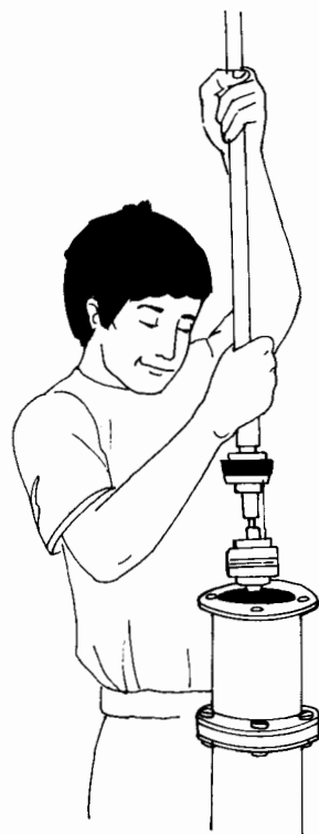
Lower footvalve and piston into cylinder
