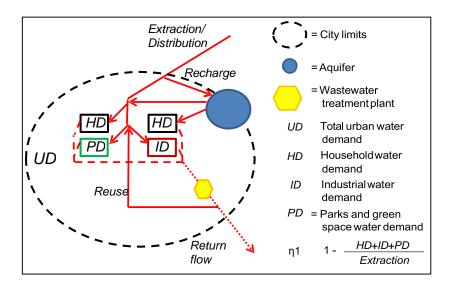
Figure 1. Simple schematic representing an urban water supply system
