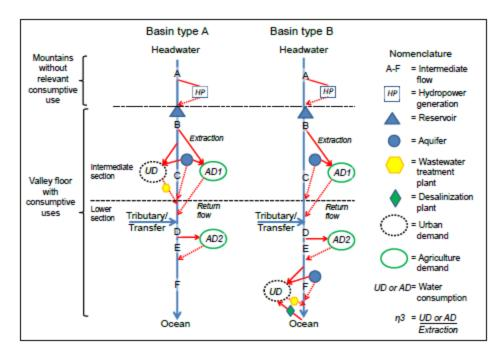
Figure 2. Schematics representing urban water supply system within a basin perspective
