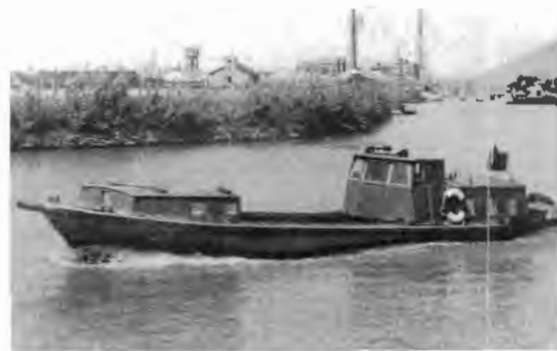
Fig. 6. A 10 000 kg (10 t), 24 hp engine, used in the waterways network of Zhejiang Province
