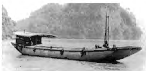
Fig. 37. A 180 000 kg (180 t) cargo barge, operates in the shallow river with cobble bed in Yueshan Region, Sichuan Province.
