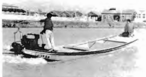
Fig. 1. An 8000-kg (8-ton), 12.67 m farmboat equipped with 12 hp engine and adjustable pitch propeller, suitable for agriculture and transport.
