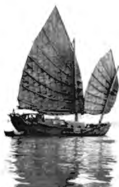
Fig. 16. The 17.1 m, 65 000 kg (65 t) dwt coastal sailing vessel with speed down of 10 knots was commissioned in Fujian and Guangdong Provinces in 1968. On July 1969 it went through a hurricane (No. 12 Beaufort Wind Scale) and heavy tidal waves for more than four hours. Its only damage was one loosen wooden bilge keel with the ferrocement hull left undamaged. The vessel has been operating quite well since then.
