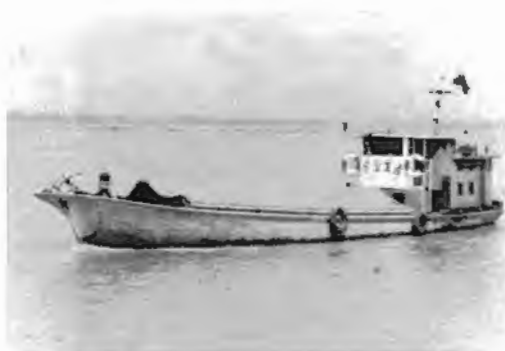
Fig. 22. "Wuhuo No. 34" is a 25 000 kg (25 t), 19.6 m LWL, 20 hp self-propelled barge in Anhui Province.
