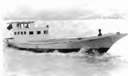
Fig. 9. A 15 dwt, LWL 16.6 m, 13.26 km/hr speed and 24 hp engine, self-propelled farm boat popular in Fuzhou City. It was produced by circular block method.
