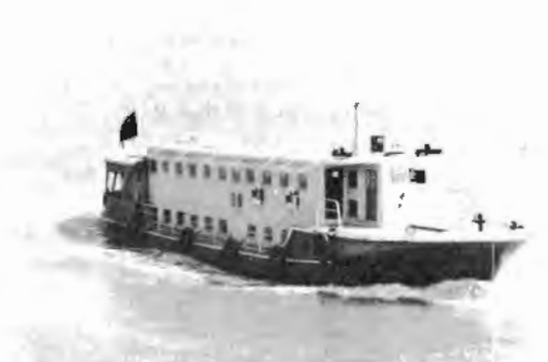
Fig. 25. A 200-person passenger ship "Xiake No. 4" has its external surface coated with epoxy-bitumen, an anti-corrosion paint. It operates between Xiamen and Shima, and also in Tongan, Fujian Province.
