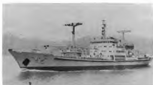
Fig. 10. The cargo ship "Gutian", China's biggest coaster ferrocement vessel (99.1 m LWL, 14.5 m moulded breadth, 8.1 m moulded width, 5 773 000 kg (5773 t) in full load displacement and 13 knots in speed) was in service in Fujian Province, carrying cargo (especially corrosive cargoes) between Chinese coastal harbors for 9 years since 1975. The hull was built with large sized thin web framing and post tensioned prestressed deck. It was produced by sectional method of hull construction, moulding of high frequency vibro-grouting.
