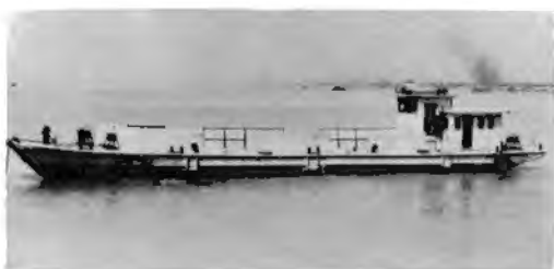
Fig. 36. A 30.5 m and 120 000 kg (120 t) payload capacity deck barge in Changjiang River.
