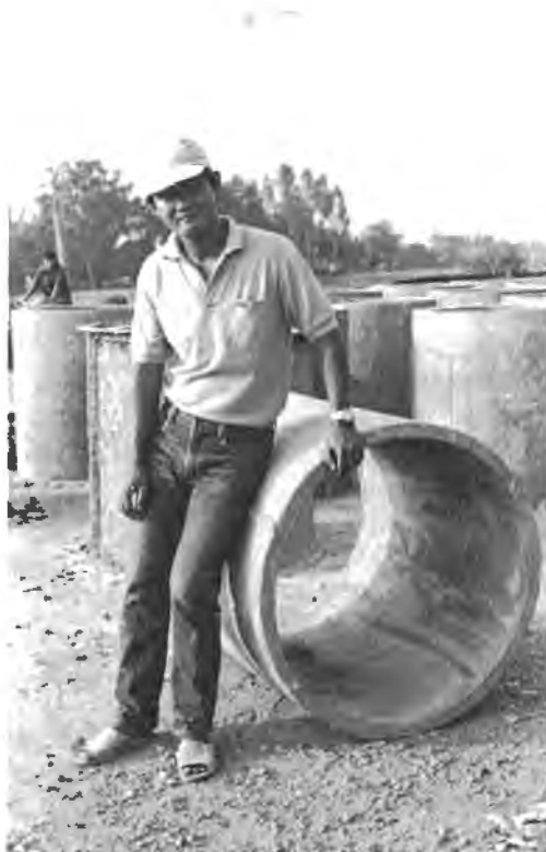
Ferrocement pipe manufactured without skeletal steel.
