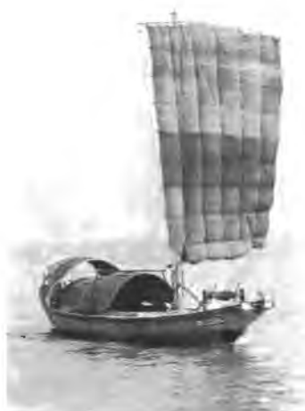
Fig. 40. A 16 m and 15 000 kg (15 t) inland river sailing vessel in the Minjiang River, Fujian Province.
