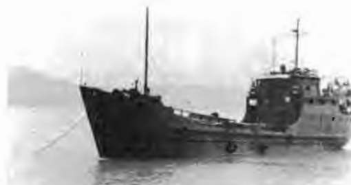
Fig. 12. "Minhai No. 167" is China's first ferrocement coaster (38.85 m LWL, 7.4 m moulded breadth, 3.7 m moulded depth, 330 dwt and 10 knots speed with a 306 hp main engine). The ship has been in operation for more than 22 years on the Fuzhou-Shanghai route and Xiamen-Hong Kong route. Its hull has not yet been overhauled and its anti-corrosion coating is still intact.
