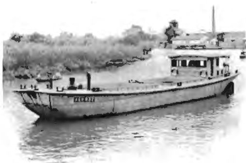
Fig. 38. A 110 000 kg (110 t) cargo barge featuring large hatch opening, operates in the inland rivers of Zhejiang Province and Changjiang River.
