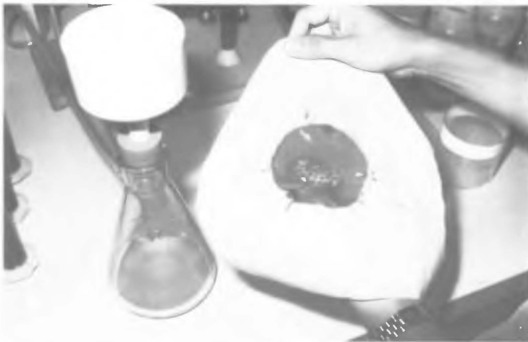
A laboratory demonstration showing the results of algae filtration on a fine-weave fabric.
