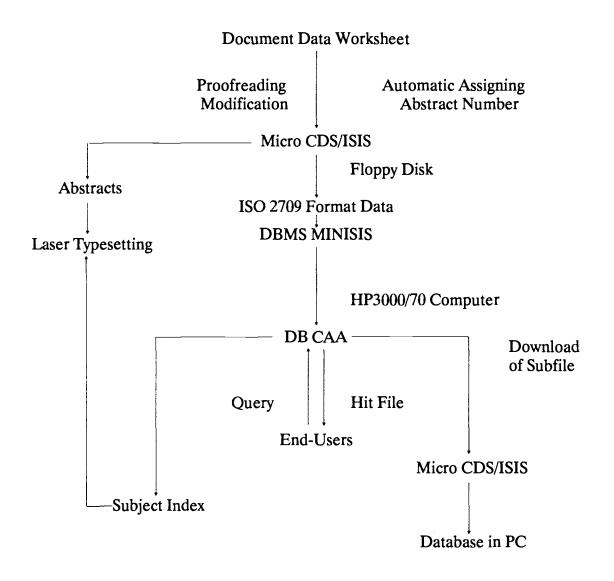
Figure 1. System Flowchart Diagram of DB CAA
