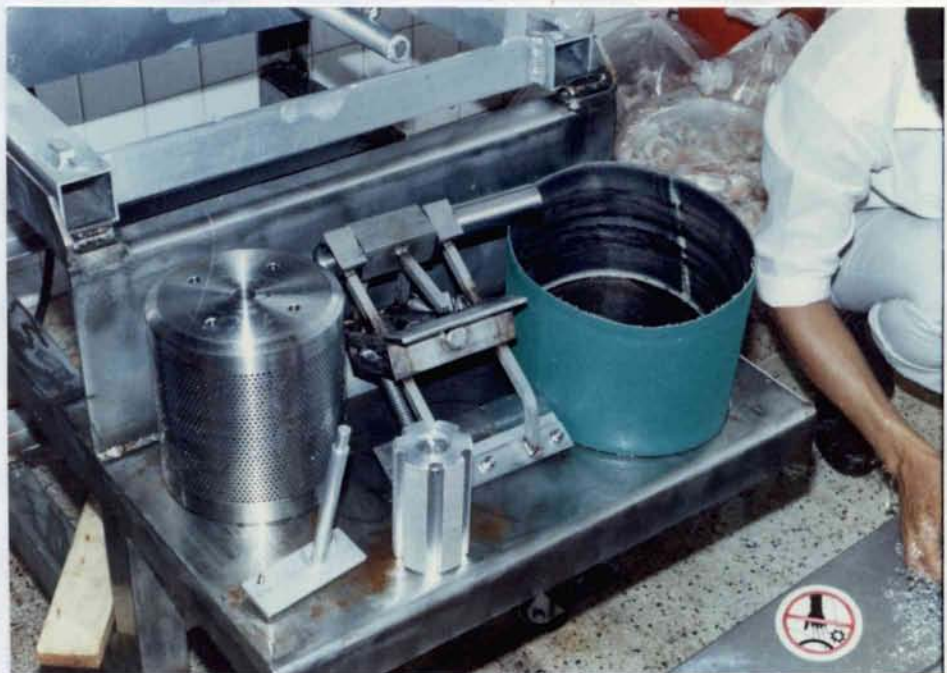
10. Major parts can be taken off for thoroughly cleaning
