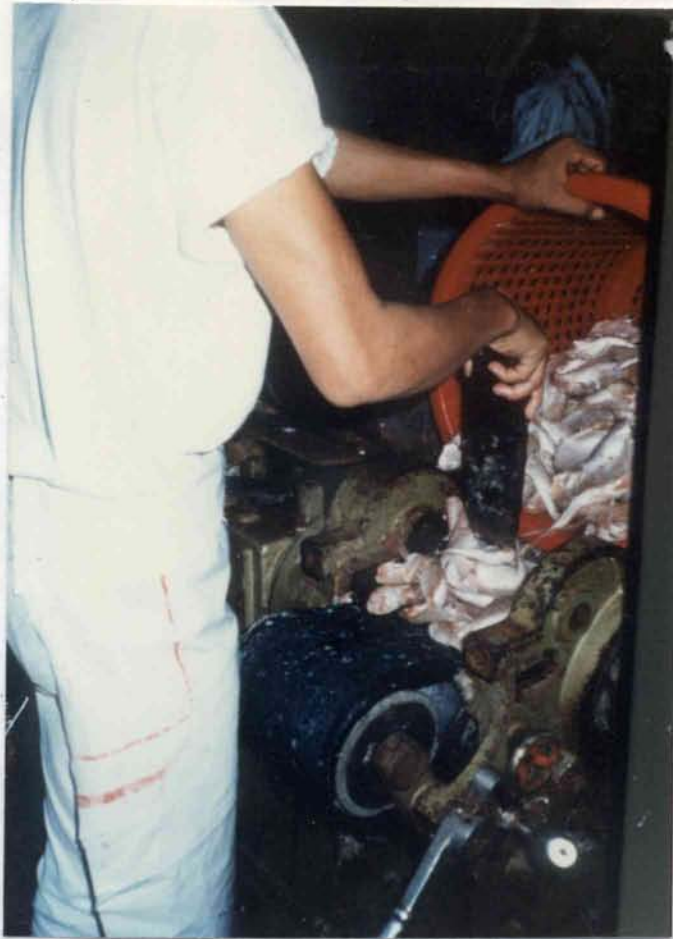
15. Feeding fish into Taiwanese commercial deboner
