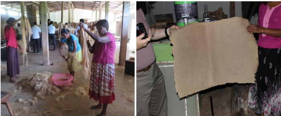
Picture showing the extraction of banana fibers and banana fiber based paper that are used in packaging industry in Sri Lanka. Over 70% of the workers in these operations are women
