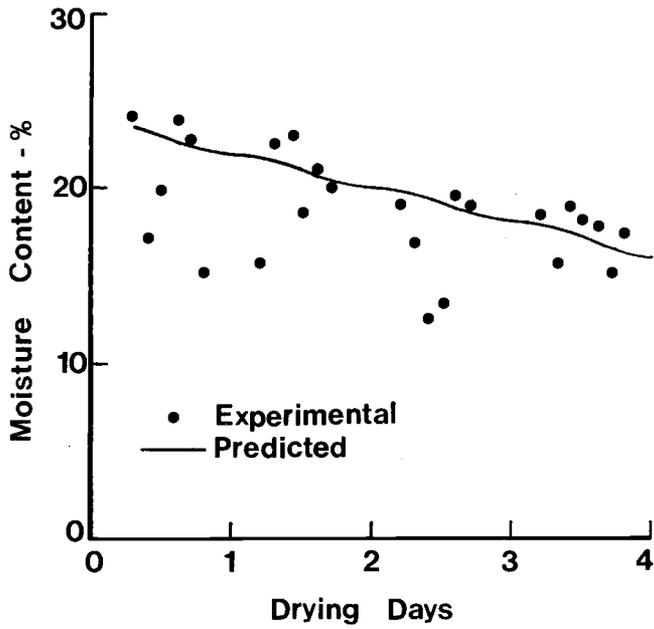
Fig. 6. Comparison of predicted and experimental results (Bassey 1982) for a rice bed thickness of 100 mm.
