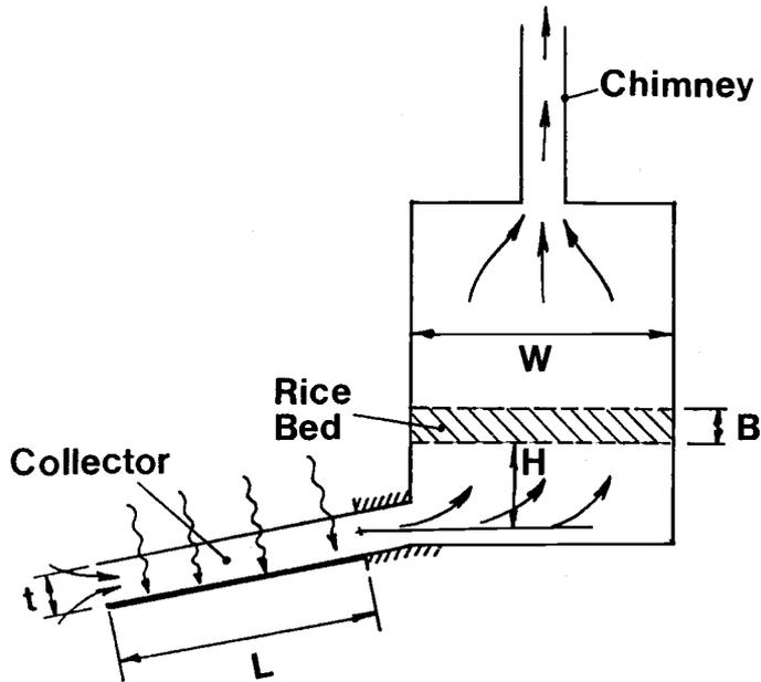
Fig. 1. Type of dryer being considered.
