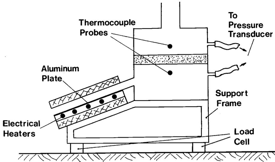
Fig. 10. Layout of experimental apparatus.
