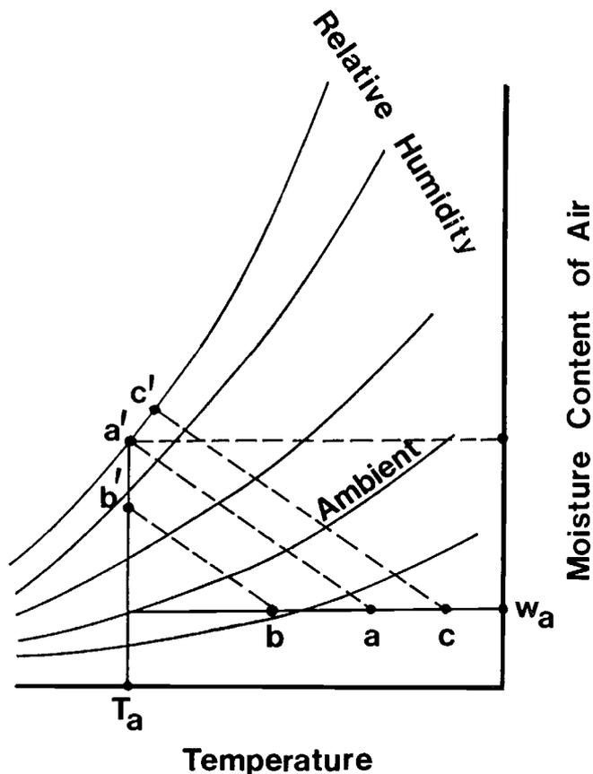
Fig. 2. Possible changes in temperature and humidity in the rice bed.
