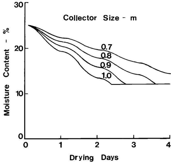
Fig. 8. Effect of collector size on dryer performance.
