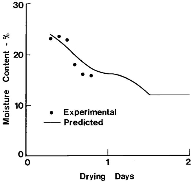
Fig. 4. Comparison of predicted and experimental results (Bassey 1982) for a rice bed thickness of 25 mm.
