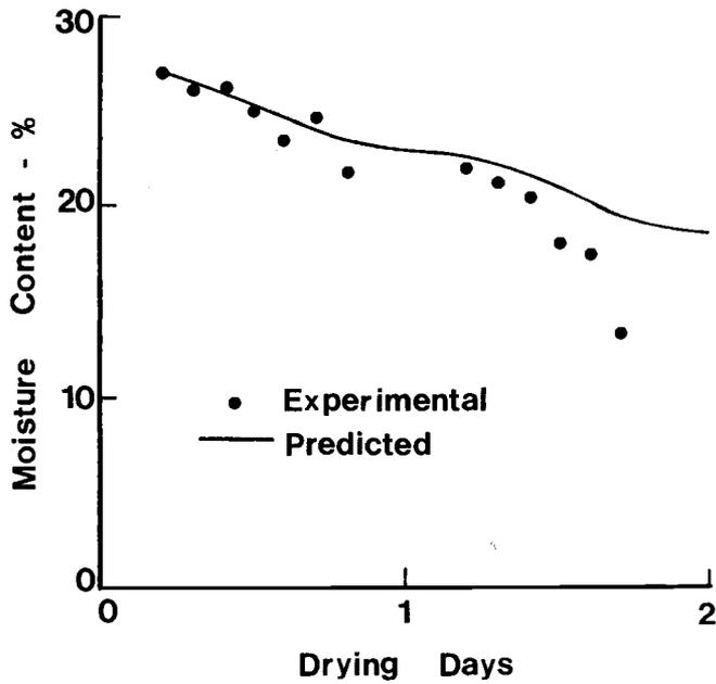
Fig. 5. Comparison of predicted and experimental results (Bassey 1982) for a rice bed thickness of 50 mm.
