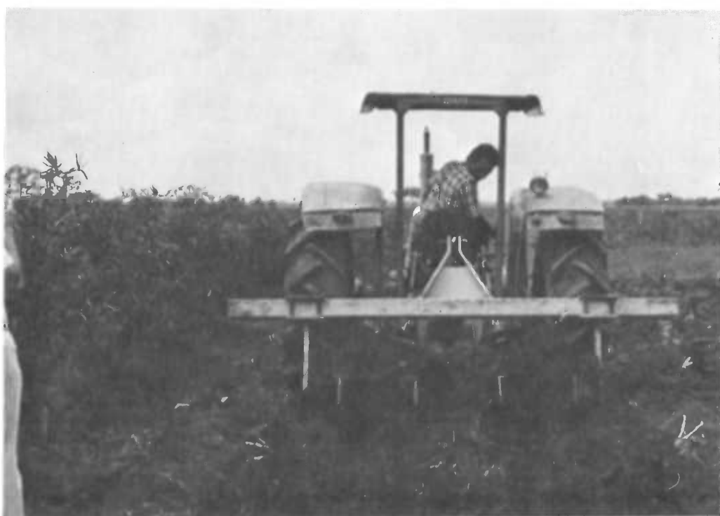
Fig. 1. The CIAT toolbar-mounted loosening blade harvests two rows of cassava at a time.
