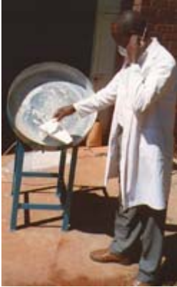
Machine for turning rock phosphate/fertilizer mixture into pellets. (Photo: P. van Straaten)
